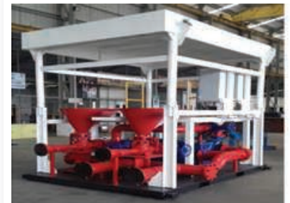
Mud Hopper on Skid
