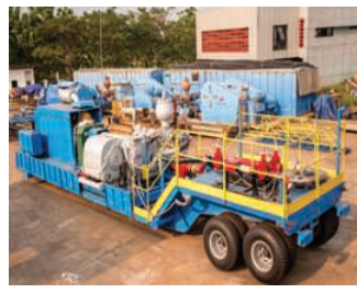
Trailer Mounted Mud Pump with Chock manifold and Poor Boy
