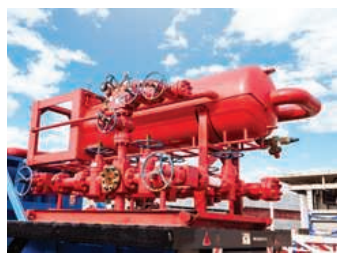
Chock Manifold and Mud Gas Separator
